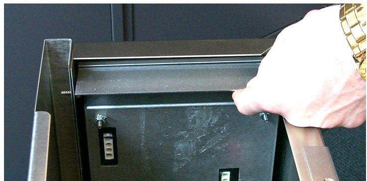
Fig.7: Position the deflector shroud on the upper mounting studs of the computer assembly.
